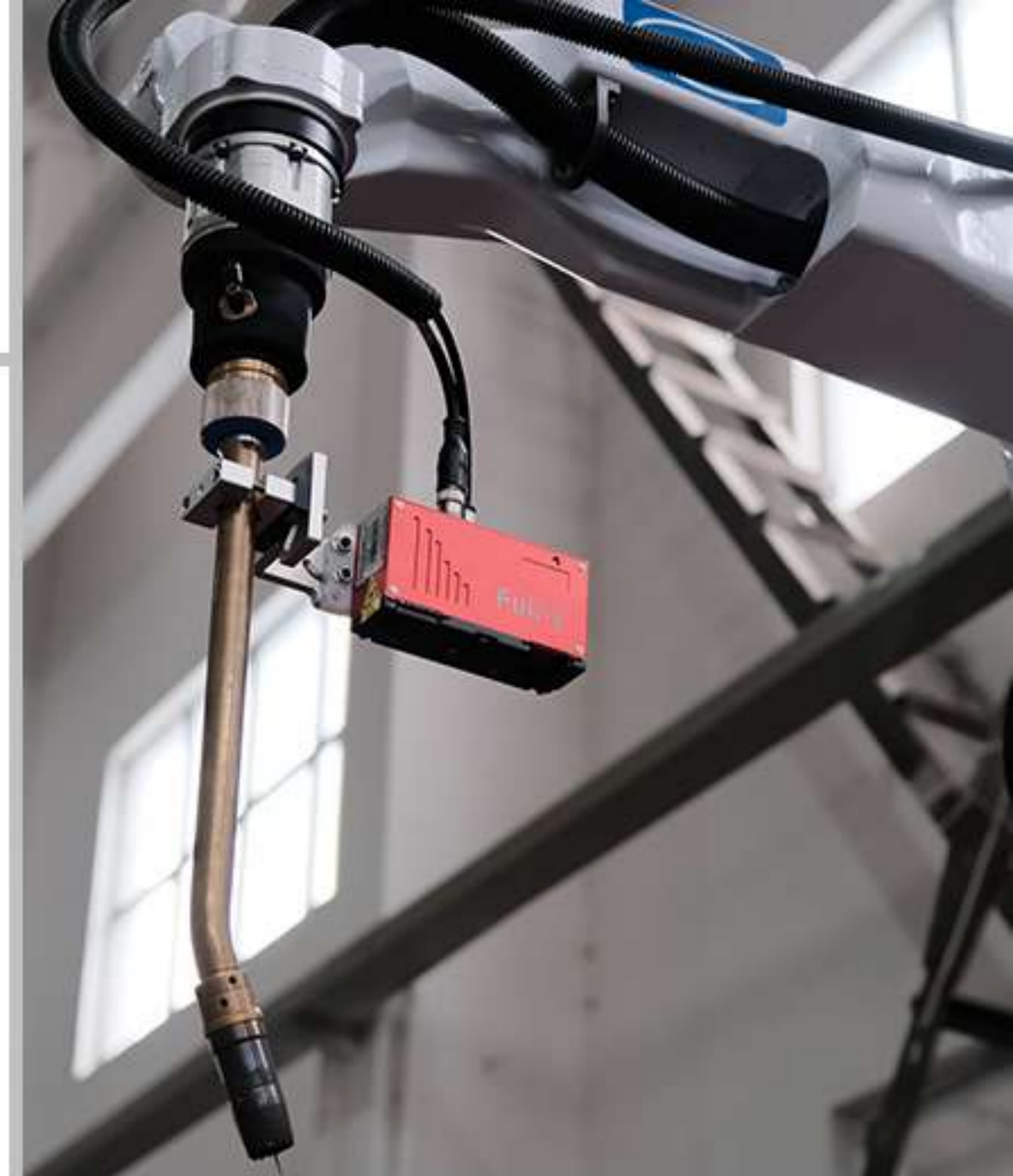
■ LASER TOUCH SENSING OF PART TO BE WELDED
